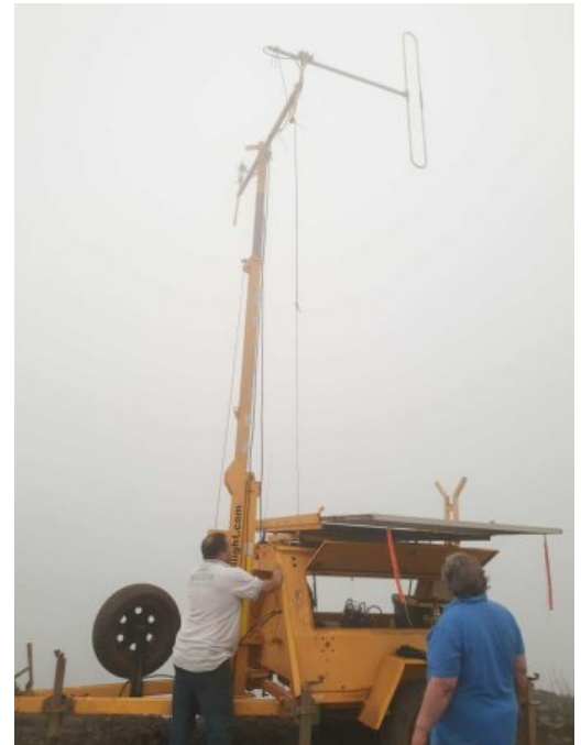
PHOTO: Radio repeater trailers were deployed to provide a radio network in the Bega area after power was lost. (Supplied: Neil Fallshaw)
