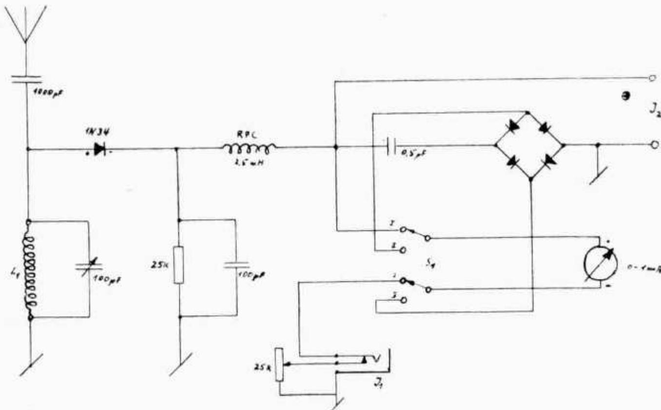
$L_1 = 28 \text{ MHz}$  3 Wdg, Dr.  $\phi$  1mm,  $\phi$  37mm, L 42mm
