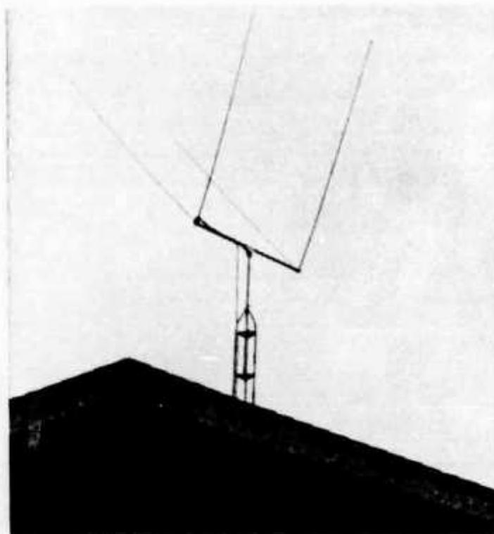
This is a 10-meter, 2-element Delta Loop that is very similar in construction to the antenna described in the article.
