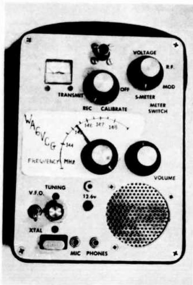
Front-panel view of the W7HCV 2-meter solid-state transceiver. The entire circuit is housed in a Simpson Model 260-style meter case. A home-made dial plate provides a frequency readout of 144 to 148 MHz.
