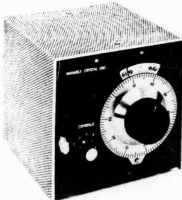
The solid-state VXO is built in a homemade aluminum cabinet. The outer cover is made of perforated stock, but can be fashioned from solid aluminum sheeting if the builder prefers the latter. Gray spray-can paint was used to finish the front and rear panels of the VXO. White press-on decals are used for labeling.
