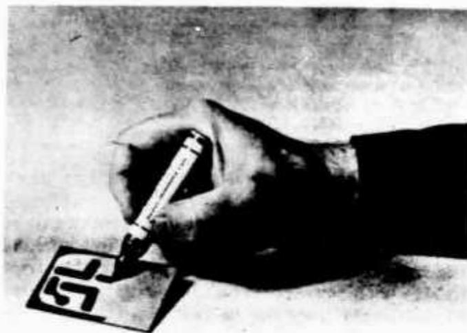
An etch-resist pen can be used to protect the retained portions of the copper foil.
