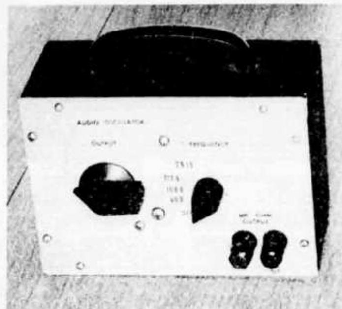
A completely self-contained source of audio test tones useful for testing and aligning equipment varying from audio amplifiers to teletype terminal units.
